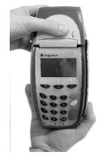
To avoid an overheating of the printer, wait a few seconds between two printings.
